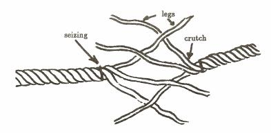
Fig. 2 shows the correct way to marry two three strand ropes before short splicing.
