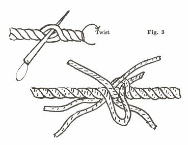
Fig. 4. To stick or tuck the strands, the first step in making a short splice.
