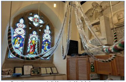
*Protective rope covers in St Margaret's, Mapledurham* conditions. Our solution was to purchase some 100 mm medium duty lay flat polythene tubing. That fits closely but not tightly over the sally. Cut into 3-metre lengths to cover the sally and hemp rope tail below it and thus provide an impervious layer around the rope and sally (*see picture on left with covers installed*). We install the covers only when we anticipate high humidity
